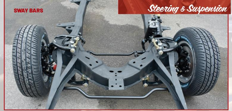
Complete Front Sway Bar Kits are heavy-duty and include all quality components. 1" bar is powder coated black and includes brackets, bushings & hardware.
