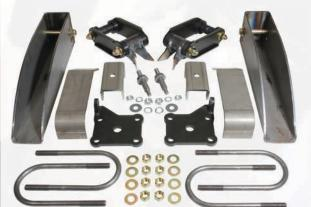
The rear spring relocation pocket kit moves your rear springs from outside the frame to underneath the frame so you are able to run 10" wide wheels without having to narrow the frame or rear-end.
