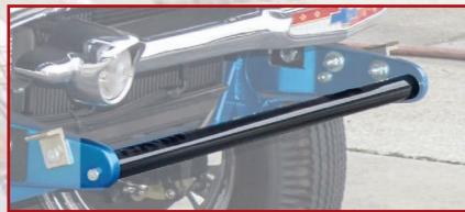
No gasser project is complete without a spreader bar up front! Originally designed as a means to skirt bumper laws back in the day, a spreader bar makes for a finished look up front when running without a factory front bumper setup. Made from 2" mild steel, these all-new spreader bars are available in raw finish or chrome plated. Available exclusively through Woody's Hot Rodz.
