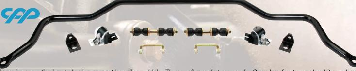
Sway bars are the key to having a great handling vehicle. They reduce body roll and help control over steer and under steer in corners. CPPs kits feature greasable poly bushings and are available in a brushed machine, black or polished finish. Available in front and rear kits for all sway bar dimensions. Black powder coated finish. Note: Protouring sway bars will not work with some
