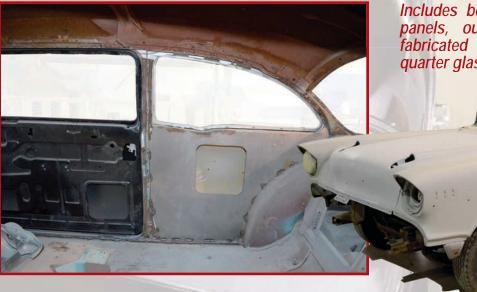
Includes both left and right full outer quarter panels, outer rockers, door shells, custom fabricated inner quarter sections, stationary quarter glass & correct window seals.
