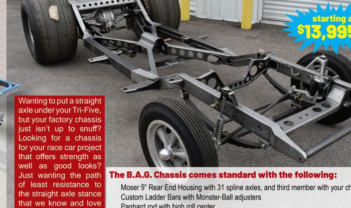
Moser 9" Rear End Housing with 31 spline axles, and third member with your choice of gearing.
