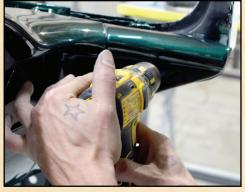
With your hole marked, use a 1/8" drill bit to make your mounting hole.
