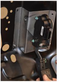
6. Cover yourself! Without a gas pedal to protrude through the firewall, you're left with a gaping hole. Woody's includes a cover and fasteners for the yoid.
