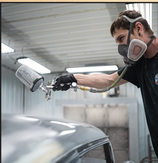
Left: One good coat of epoxy primer goes down before the 2K primer is sprayed. This is the base of the rest of your paint job, so be sure you have full coverage on all parts to have primer sprayed on them.
