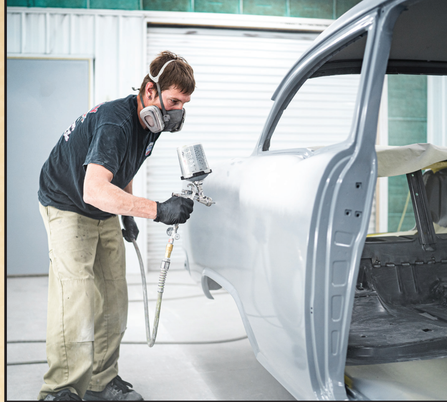
Spraying the epoxy primer on the whole car before the final primer is sprayed. This helps the primer adhere to the spots I have sanded to bare metal. Spraying the whole car ensures I will not have any dry spots on the primer to sand out before paint.
