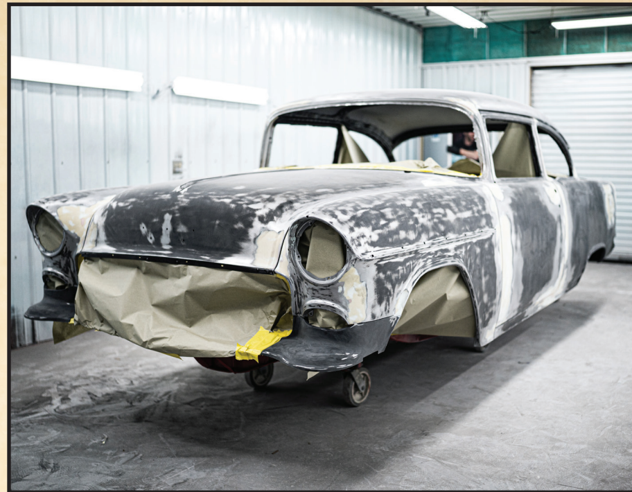
Top: Here you see the car straight out of the body shop into the paint booth, preparing for the first prime.
