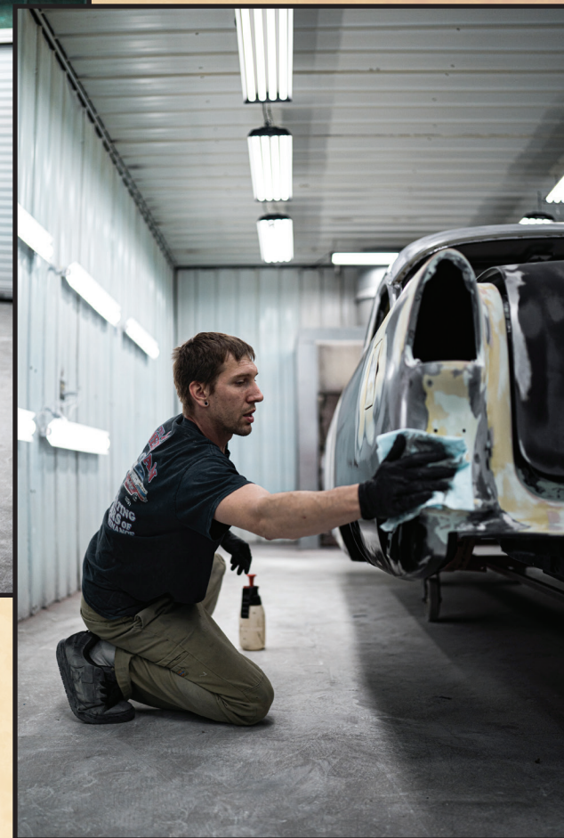
Right: One big step before any material is sprayed onto the car, pre-clean. A good wax and grease remove with low-lint towels will go a long way.
