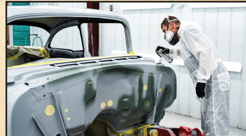
Yes, I know, looks like I sanded through a lot here with all the etch primer on the firewall. But, keep in mind, new firewall equals only one prime. That one coat of primer is not very thick on those edges, so the metal comes through faster than you think.
