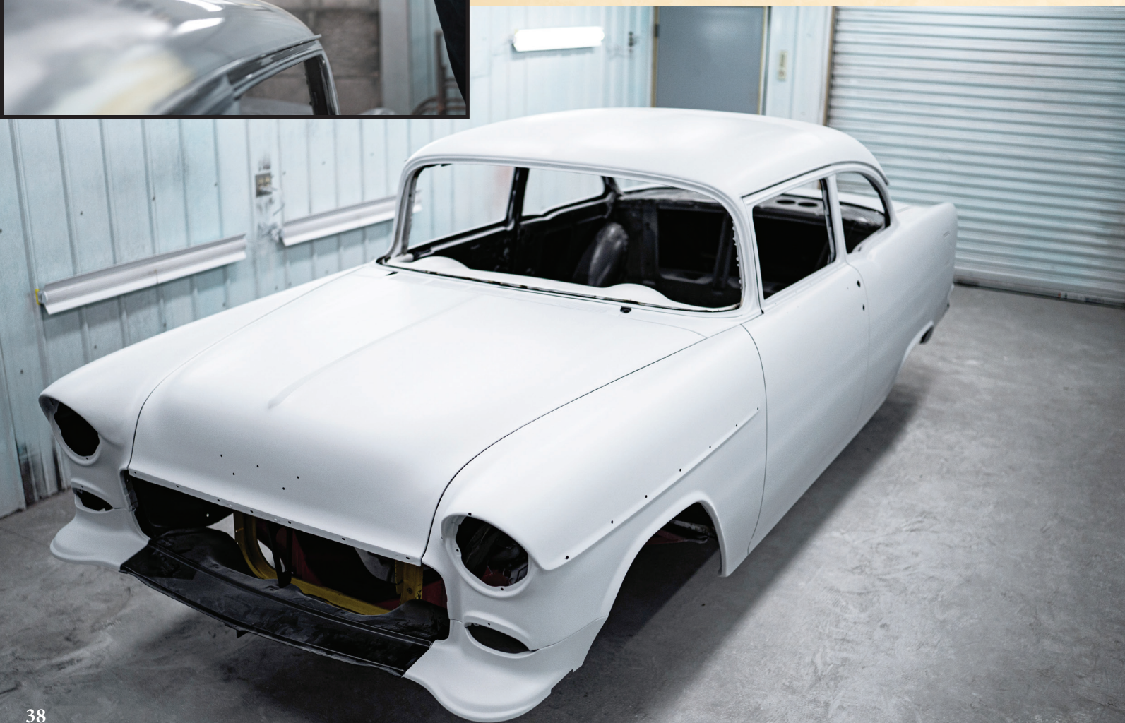
Left: One good coat of epoxy primer goes down before the 2K primer is sprayed. This is the base of the rest of your paint job, so be sure you have full coverage on all parts to have primer sprayed on them.
